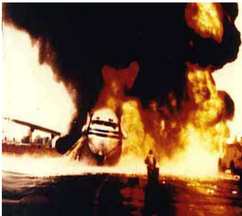
The aircraft caught fire after a fuel line was severed during its takeoff roll. The takeoff was successfully aborted, and all occupants were evacuated.
